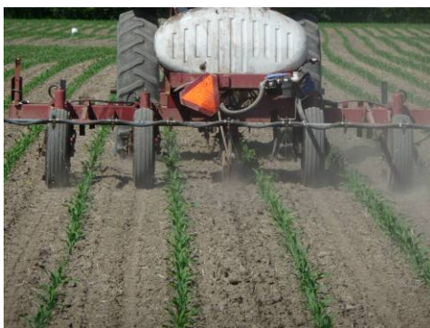
Figure 2: Post Emergent Broadcast Application of UAN to Standing Corn Using Streamer
