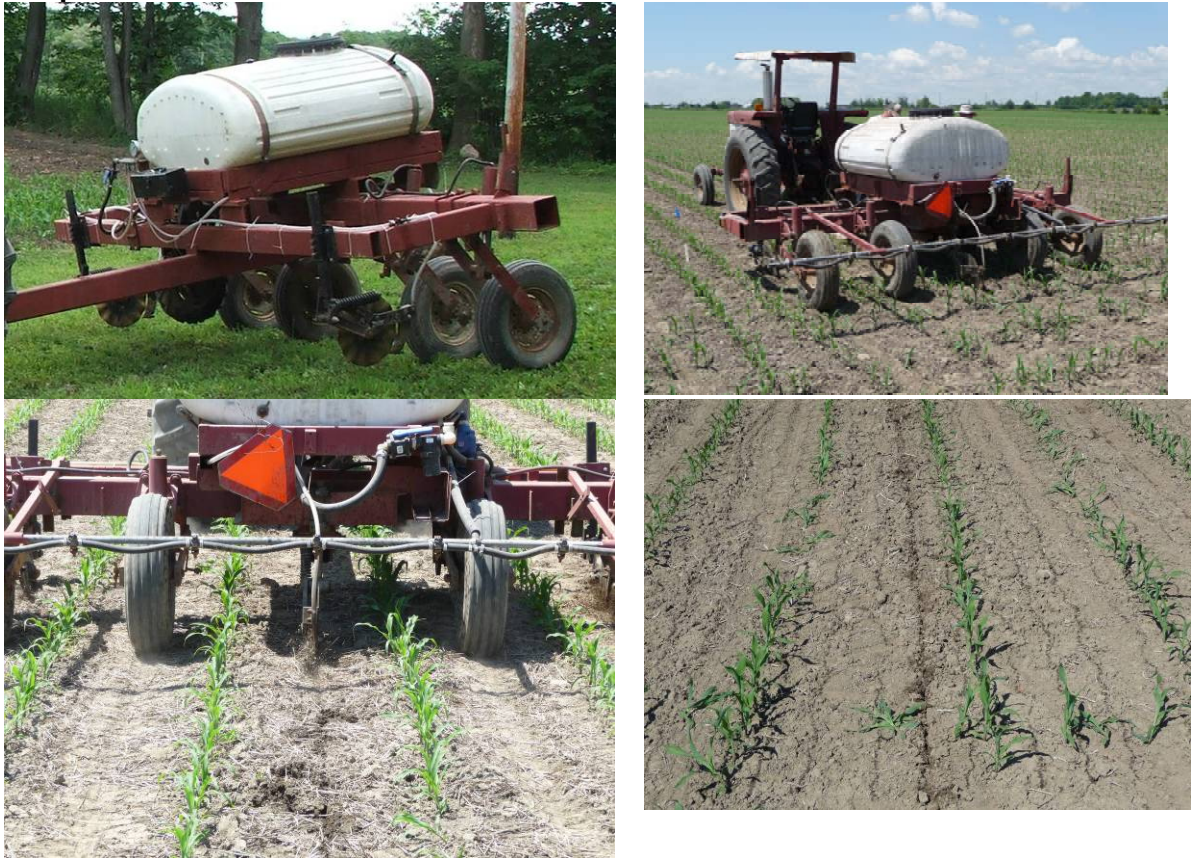
Figure 2: Post Emergent Broadcast Application of UAN to Standing Corn Using Streamer
